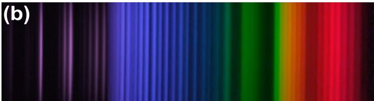
Figure 5 -- (a) Diagram of the full optical setup. (b) The resulting spectrum. This spectrum is stitched together between the UV and visible parts with the UV false-colored.
